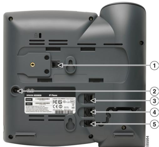
**CAUTION** Do not insert a telephone line cord into the port marked "AUX" (1).
